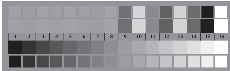
Picture B3: 14 CIE-test colours and 2 + 16 grey steps; Use of PS operator cmy0*/000n* setcmykcolor
