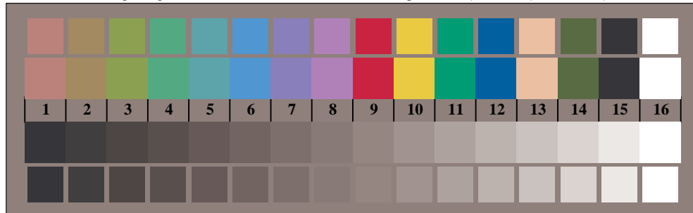
Picture D3: 14 CIE-test colours and 2 + 16 grey steps; Use of PS operator cmy0* setcmykcolor (only)
