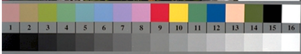
Picture D1: Flower motif, 14 CIE-test colours and 2 + 16 grey steps (nf); PS operators settransfer , 3 colorimage
