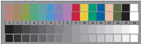
Picture D3: 14 CIE-test colours and 2 + 16 grey steps; Use of PS operator olv* setrgbcolor (only)
