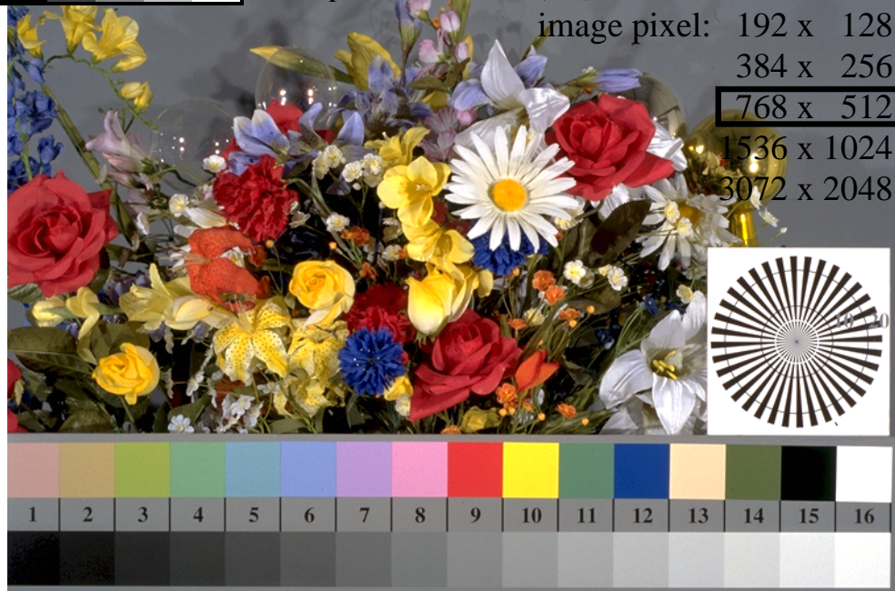
Picture B1: Flower motif, 14 CIE-test colours and 2 + 16 grey steps (sf); PS operators settransfer , 3 colorimage
