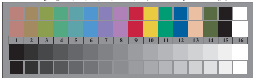
Picture B3: 14 CIE-test colours and 2 + 16 grey steps; Use of PS operator olv* setcolor / w* setgray
