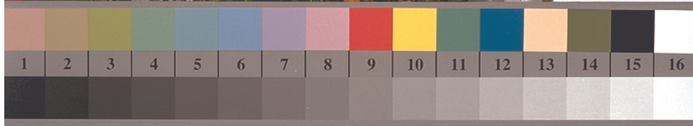
Picture D1: Flower motif, 14 CIE-test colours and 2 + 16 grey steps (nf); PS operators settransfer , 4 colorimage
