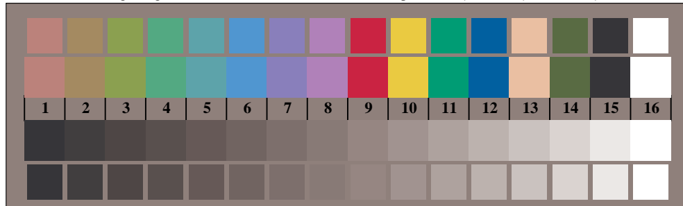
Picture D3: 14 CIE-test colours and 2 + 16 grey steps; Use of PS operator cmY0* setcmYcolor (only)
