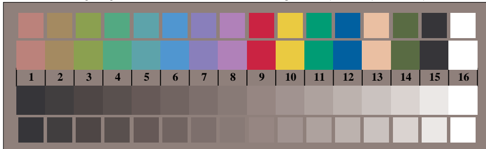
Picture D3: 14 CIE-test colours and 2 + 16 grey steps; Use of PS operator cmly0* setcmlycolor (only)
