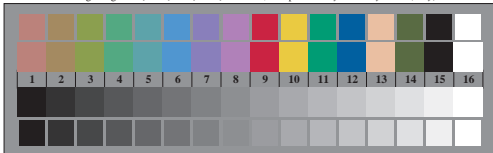
Picture D3: 14 CIE-test colours and 2 + 16 grey steps; Use of PS operator cmy0* setcmkcolor (only)
