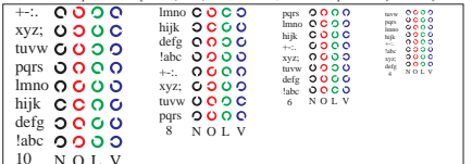
Picture D5: Script and Landolt-rings N, O, L and V; Use of PS operator cmy0* setcmkcolor (only)
