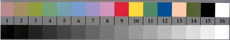
Picture D1: Flower motif, 14 CIE-test colours and 2 + 16 grey steps (nf); PS operators settransfer , 3 colorimage
