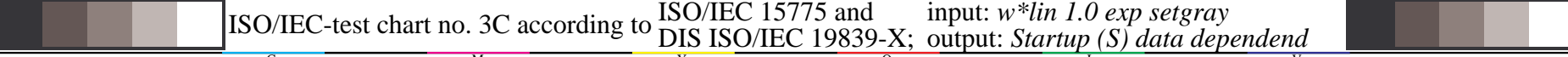
Picture C3: 16 visual equidistant L^* -grey steps; PS operator: w*lin 1.0 exp setgray
