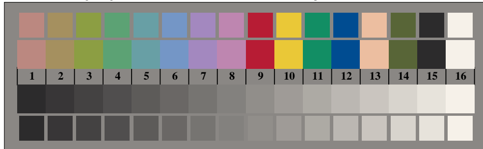
Picture B3: 14 CIE-test colours and 2 + 16 grey steps; Use of PS operator LAB* setcolor
