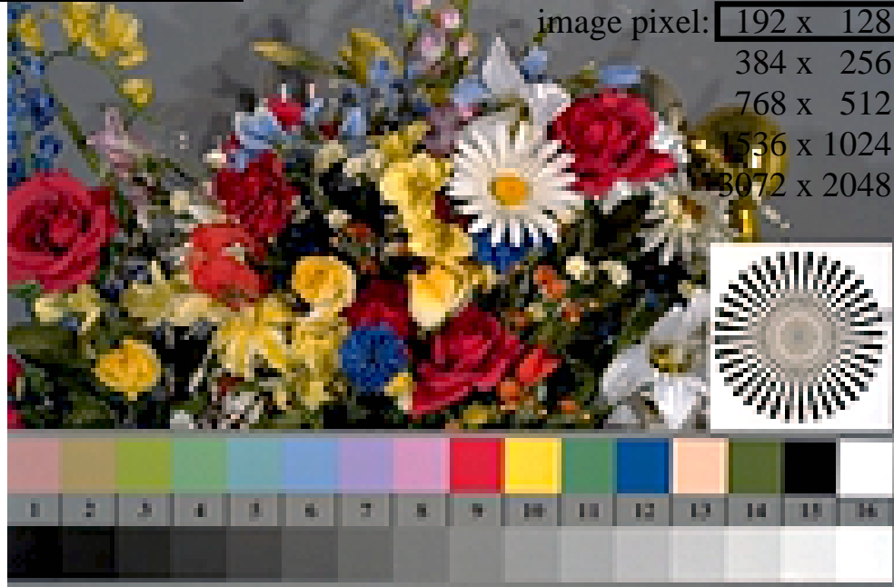
Picture D1: Flower motif, 14 CIE-test colours and 2 + 16 grey steps (nf); PS operators settransfer , 3 colorimage
