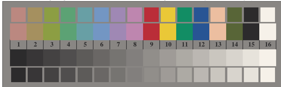
Picture B3: 14 CIE-test colours and 2 + 16 grey steps; Use of PS operator olv* setrgbcolor / w* setgray
