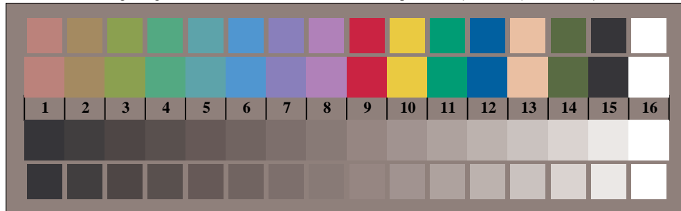
Picture D3: 14 CIE-test colours and 2 + 16 grey steps; Use of PS operator cmY0* setcmykcolor (only)
