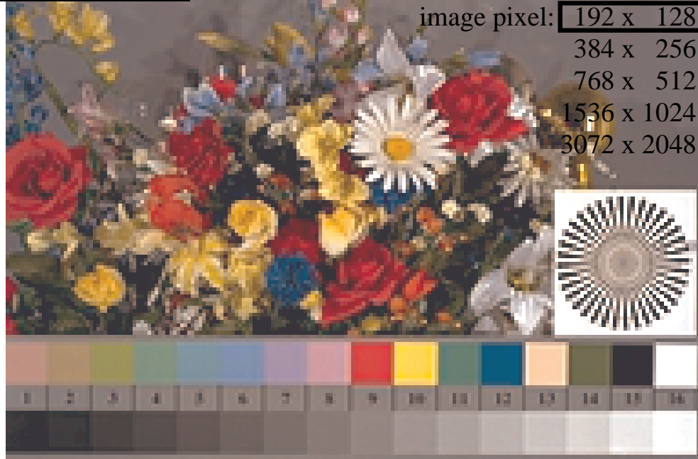
Picture D1: Flower motif, 14 CIE-test colours and 2 + 16 grey steps (nf); PS operators settransfer , 4 colorimage
