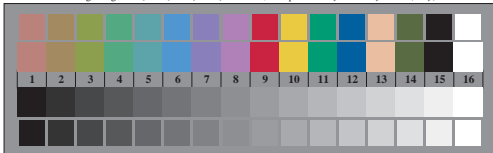
Picture D3: 14 CIE-test colours and 2 + 16 grey steps; Use of PS operator cmy0* setcmycolor (only)
