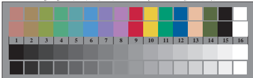
Picture D3: 14 CIE-test colours and 2 + 16 grey steps; Use of PS operator olv*setgrbcolor (only)
