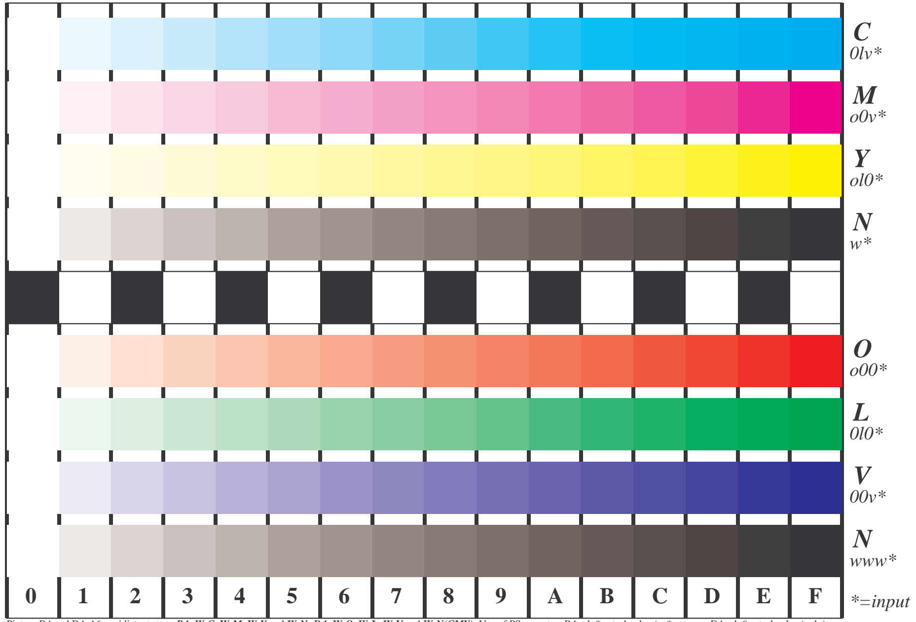
Picture B4 and D4: 16 equidistant steps B4 : W-C, W-M, W-Y and W-N; D4 : W-O, W-L, W-V and W-N(CMY); Use of PS operator; B4 : olv* setrgbcolor / w* setgray ; D4 : olv* setrgbcolor (only)
