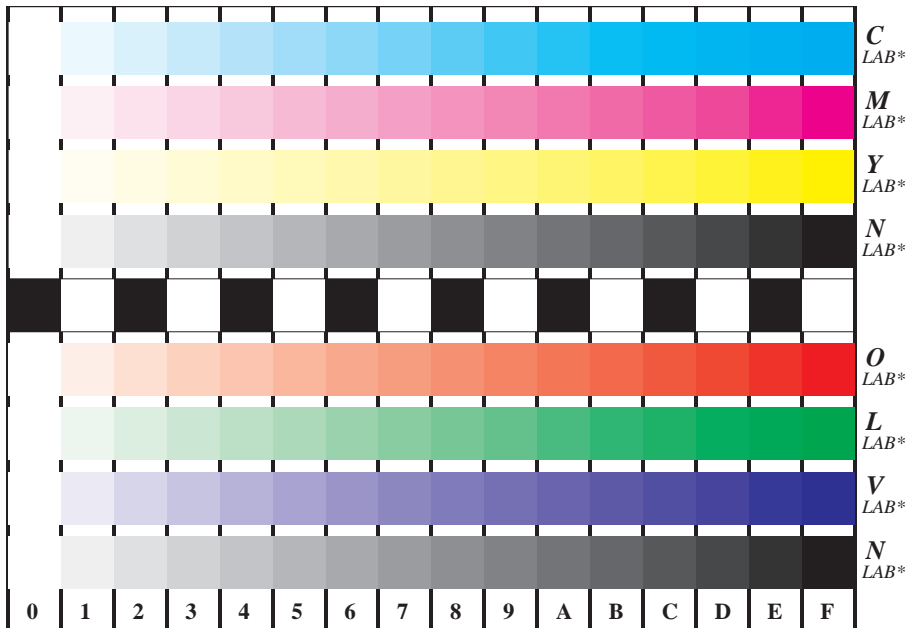
Figure B4 and D4 of the ISO/IEC-test charts no. 2 and 4; 16 visual equidistant steps of colour series; Use of the PS operator LAB* setcolor
