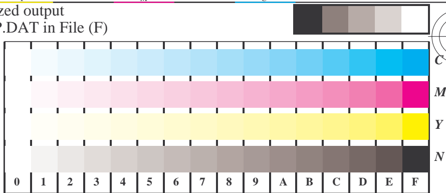
Picture B4w: 16 equidistant steps W-C, W-M, W-Y and W-N; PS operator cm\gamma0^* setcmykcolor (only)
