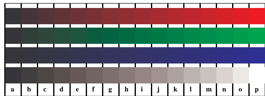
Picture D4n: 16 equidistant steps N-O, N-L, N-V and N-W ; PS operator cmY0* setcmykcolor (only)
