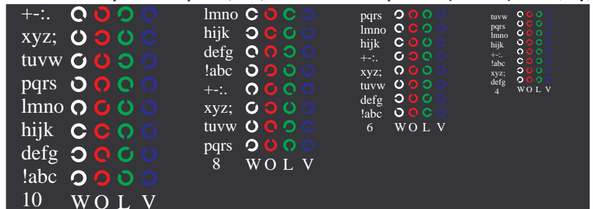
Picture D5n: Script and Landolt-rings W , O , L and V ; PS operator cmY0* setcmykcolor (only)
