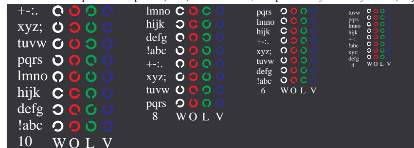
Picture D5n: Script and Landolt-rings W , O , L and V ; PS operator cm\dot{y}0^* setcmykcolor (only)
