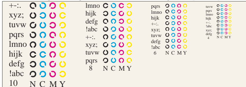
Picture B5w: Script and Landolt-rings N, M, C and Y; PS operator cmy0* setcmykcolor (only)
