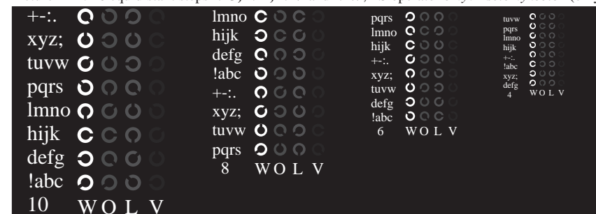
Picture D5n: Script and Landolt-rings W, O, L and V ; PS operator cmy0* setcmykcolor (only)
