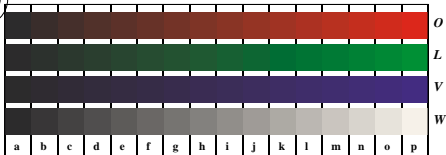
Picture D4n: 16 equidistant steps W-O, W-L, W-V and W-N; PS operator LAB* setcolor
