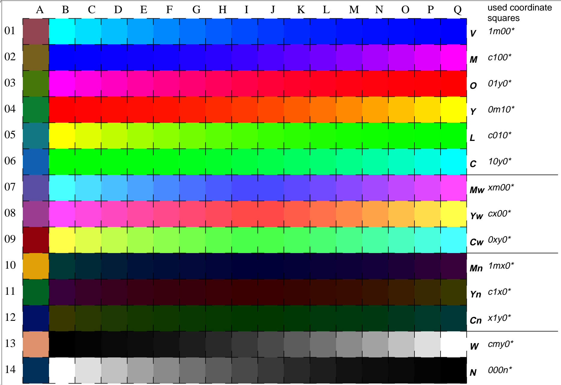
16 equidistant CIELAB steps in cmy0*(TLS00) for colour series C-V, V-M, M-O, O-Y, Y-L, L-C, N-W, W-N, Cw-Mw, Mw-Yw, Yw-Cw, Cn-Mn, Mn-Yn, Yn-Cn and 14 CIE-test colours (left)
