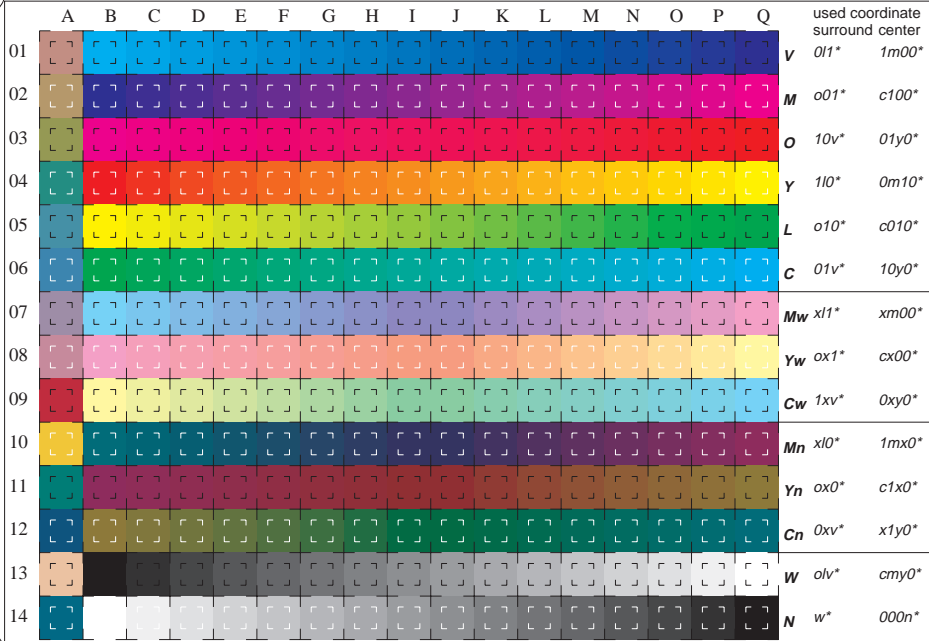
16 equidistant CIELAB steps in olv^*(TLS00) , cmy0^*(TLS00) for colour series C-V, V-M, M-O, O-Y, Y-L, L-C, N-W, W-N, Cw-Mw, Mw-Yw, Yw-Cw, Cn-Mn, Mn-Yn, Yn-Cn and 14 CIE-test colours (left)
