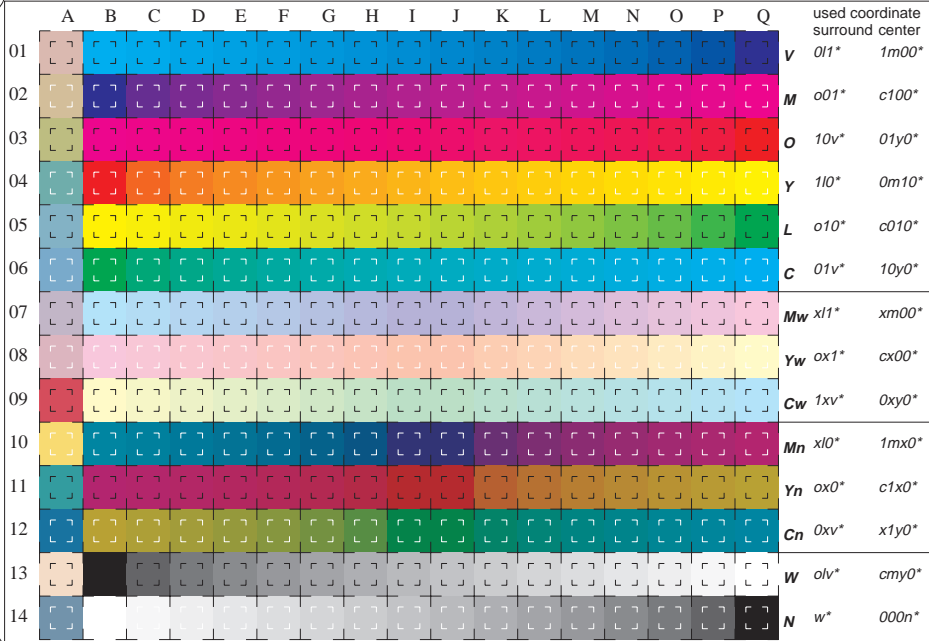
16 equidistant CIELAB steps in olv° (T LS00 ), cmv0° (T LS00 ) for colour series C-V, V-M, M-O, O-Y, Y-L, L-C, N-W, W-N, Cw-Mw, Mw-Yw, Yw-Cw, Cn-Mn, Mn-Yn, Yn-Cn and 14 CIE-test colours (left)
