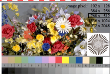
AGE20-1N, Picture 01: Flower motif, 10 CIE test colours and 16 grey steps (d), PI operators \text{rgb} \rightarrow \text{rgb}_{\text{L}} , \text{L} \rightarrow \text{rgb}_{\text{L}}
