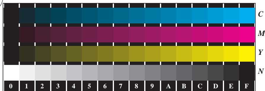
Fe010-1, Picture B4N: 16 equidistant steps N-C, N-M, N-Y, W-N; PS operator olv* setrgbcolor
