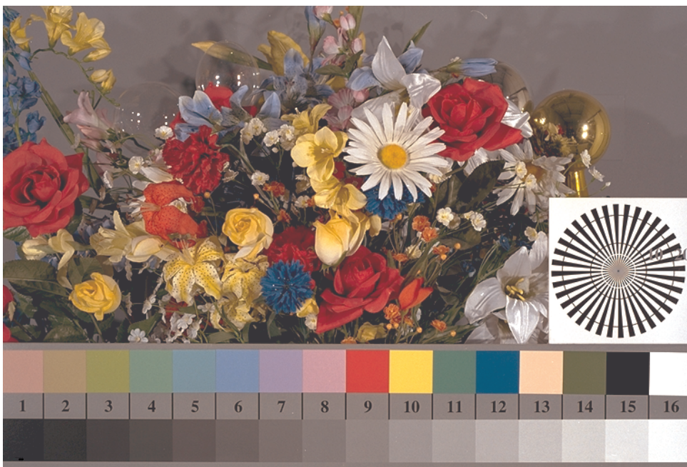
Fe020-3, Picture B1: Flower motif, 14 CIE-test colours, 16 grey steps (nf); PS operators settransfer , 4 colorimage
