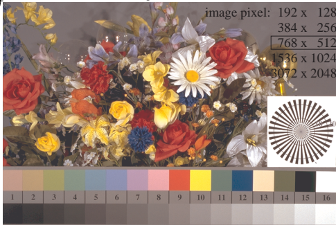
Fe040-3, Picture B1: Flower motif, 14 CIE-test colours, 16 grey steps (sf), PS operators settransfer , 4_colorimage
