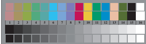
Fe070-7, Picture B3: 14 CIE-test colours and 2 + 16 grey steps; Use of PS operator oly* setrgbcolor
