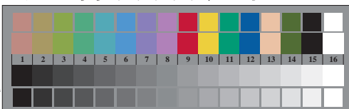
Fe490-7, Picture B3: 14 CIE-test colours and 2 + 16 grey steps; Use of PS operator olv* setrgbcolor
