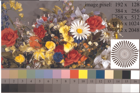
Fe490-3, Picture B1: Flower motif, 14 CIE-test colours, 16 grey steps (st); PS operators settransfer , 4 colorimage
