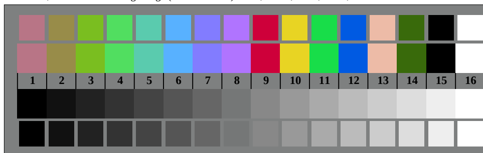
DEE00-7, Picture B3: 14 CIE-test colours according to CIE 13.3 and 16 grey steps
