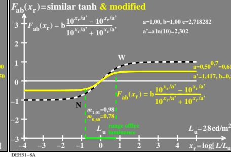
TUB-test chart DEH5; Model of response functions  $F_{ab}(x_r)$  and deviations  $\tanh(x_r)$  and deviations with  $e^{x_r/a}$  and  $10^{x_r/a}$ ;  $a^n=a^{0,7}$
