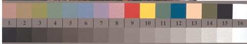
IE860-3, Picture B1: Flower motif, 14 CIE-test colours, 16 grey steps (nf); PS operators settransfer , 4 colorimage
