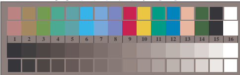
IE860-7, Picture D3: 14 CIE-test colours and 2 + 16 grey steps; Use of PS operator ohv* setrgbcolor
