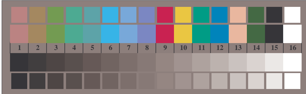
IE860-7, Picture D3: 14 CIE-test colours and 2 + 16 grey steps; Use of PS operator olv* setrgbcolor
