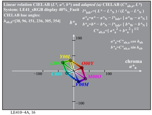
Fig. 8 — Linearized device colours of sRGB device for luminance reflections  $L_r = 0\%$ ,  $2,5\%$ , and  $40\%$
