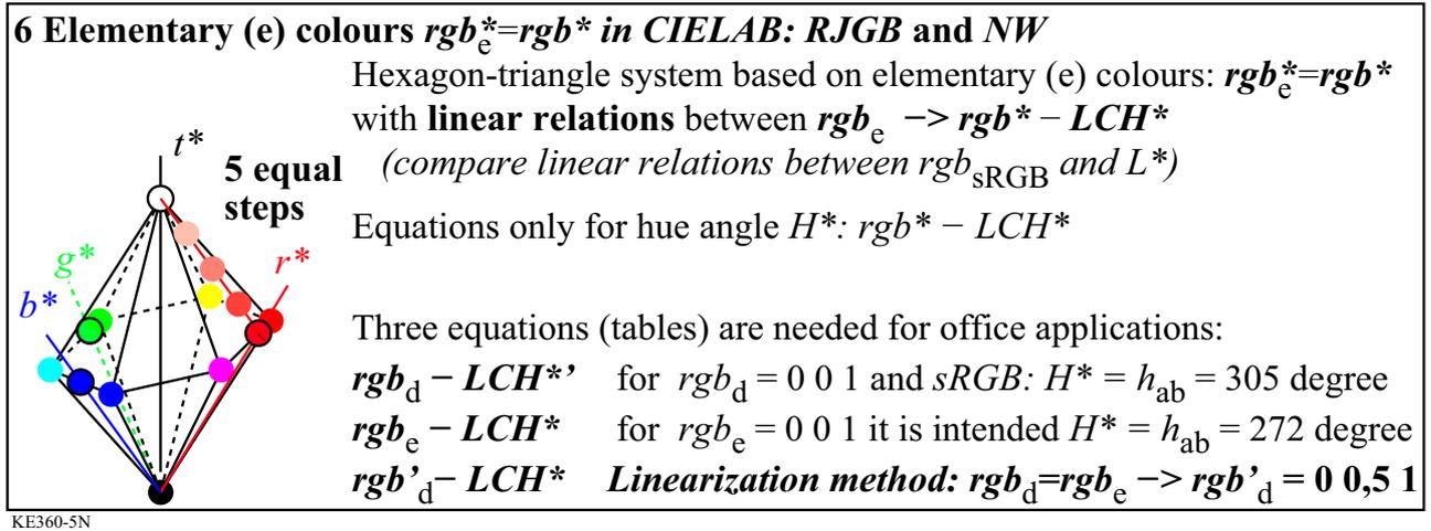
Fig. 2 — Output linearization for device and elementary colours of maximum CIELAB chroma  $C^*_{ab}$
