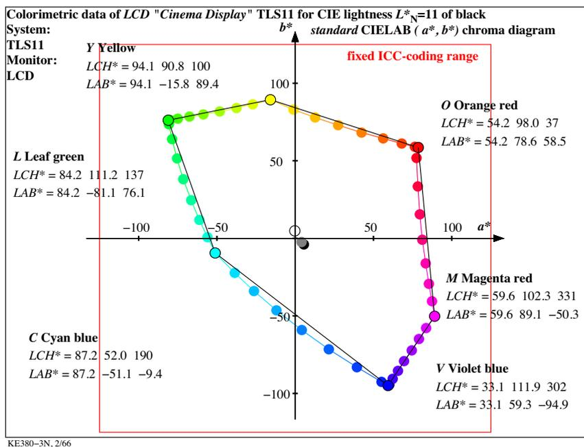
Fig. 5 — Measurement data of a LCD display for  $L_r=1\%$  ( $L^*=11$ ) in a CIELAB ( $a^*, b^*$ )-chroma plane
