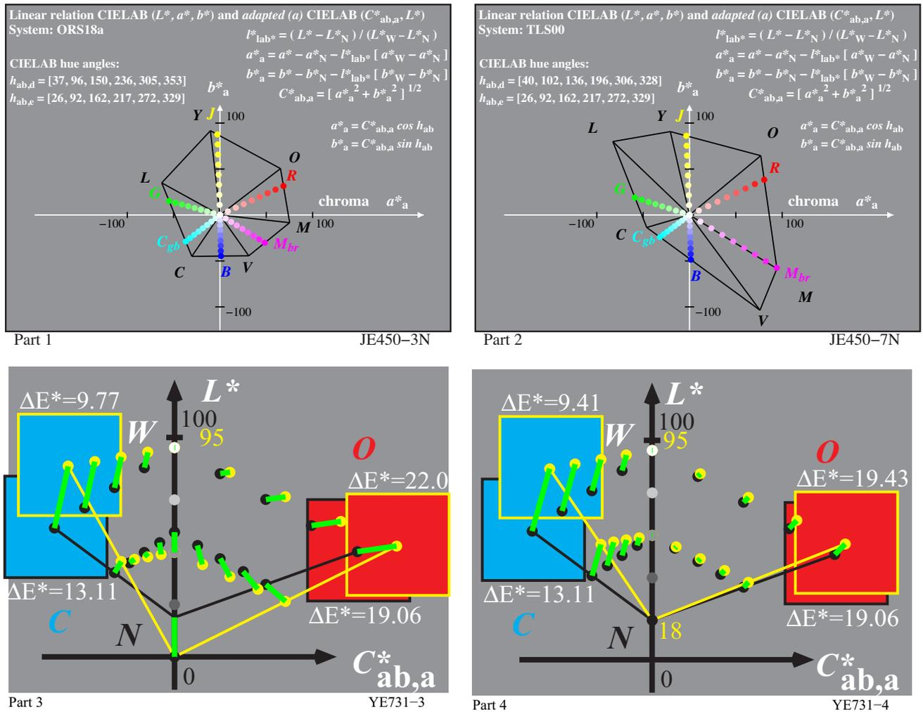
Fig. 6 — Device and elementary colours and affine transformation for three device systems
