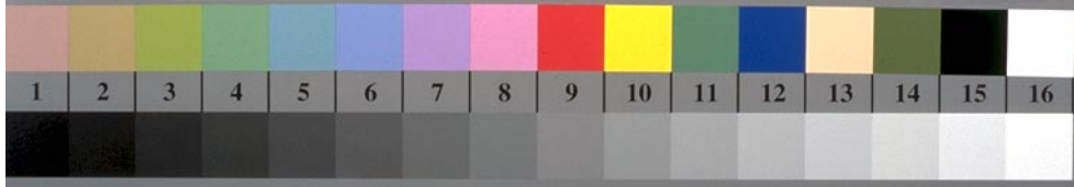
OE580-7, Picture B1-030-0: Flower motif, 14 CIE-test colours and 2 + 16 grey steps (sf); PS operators settransfer , 3 colorimage
