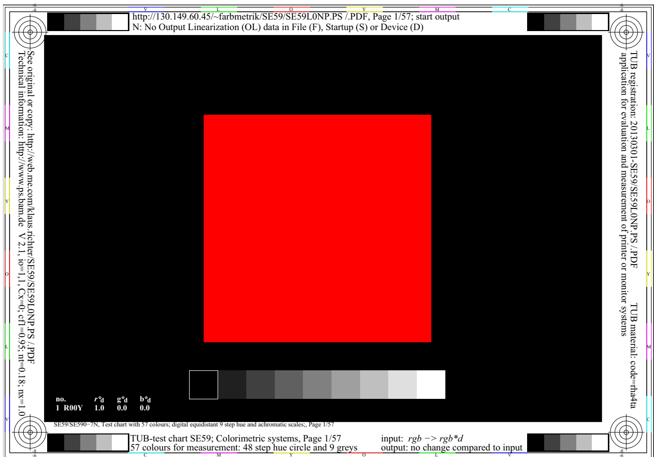
Fig D.1 — Display output for colour measurement of a 48 step hue circle and 9 grey steps
