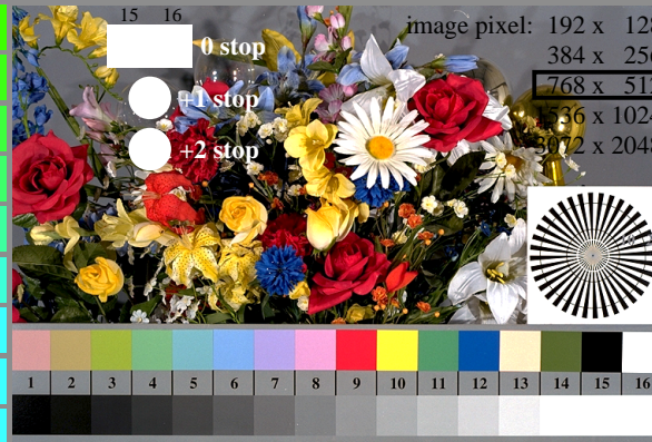
fen20-7N, Picture B1-130-2: Flower motif, 14 CIE-test colours and 2+16 grey steps (nD); PS operators settransfer, 3 colorimage
