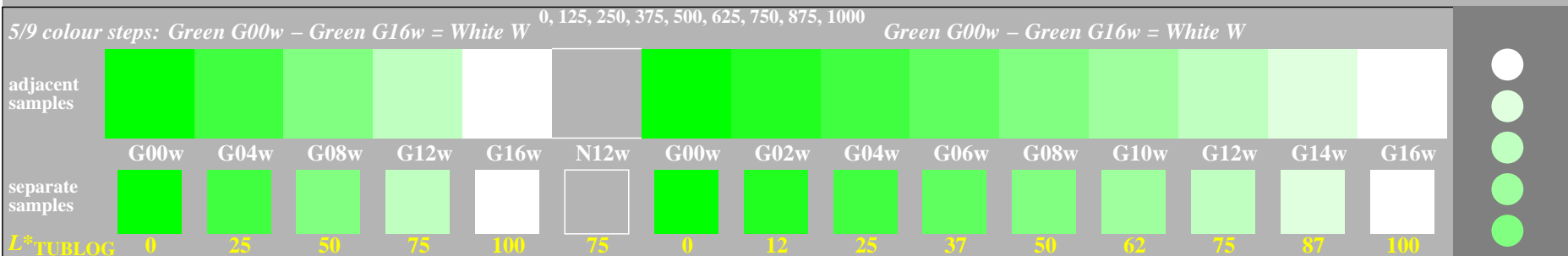
TUB-test chart gee8; Adjacent and separate colour samples for intervall scaling Evaluation of colour steps of the series G–W with 5 and 9 steps; surround light Grey H=N12w
