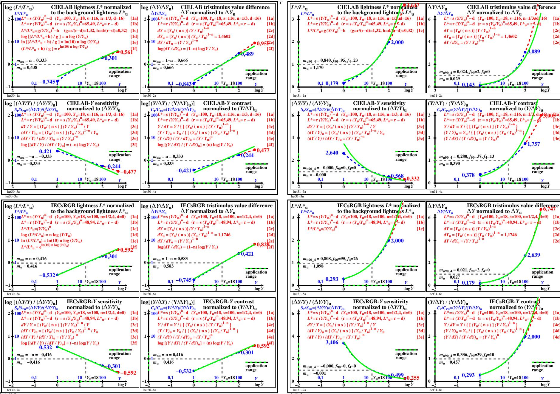
TUB-test chart het3; CIELAB & IECsRGB colour-difference, ISO/CIE 11664-4 & IEC 61966-2-1
