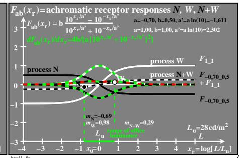
TUB-test chart hev4; Model responses  $F_{ab}(x_r)$ , processes N ( $-1 < a < -0.7, b=0.5$ ), W ( $a=b=1$ ), N+W, and derivations Tangens hyperbolicus  $\tanh(x_r)$  and modified with  $e^{\pm x_r/a}$  and  $10^{\pm x_r/a}$ ;  $a' = a \ln(10)$ ; no (+0,5)-shift
