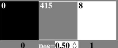
The gamma value  $\gamma_{inv}=1,000$  of the software *GammaAdjuster* reaches equal differences and corresponds to  $p_{08}=0,50$ .
